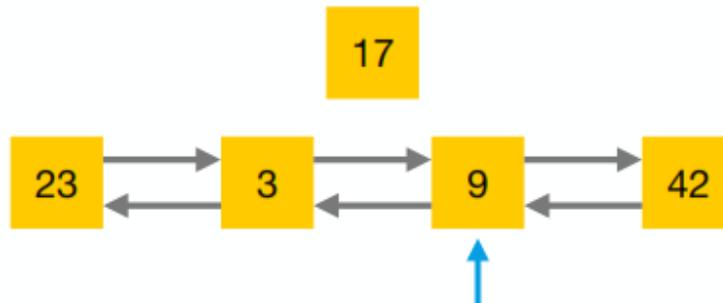
The backlink from "9" to "3" is removed and replaced with a backlink to the new element, "17".
