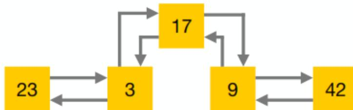
Removing an element from a doubly-linked list follows the same steps as when we insert an element into the list, just in reverse order.
