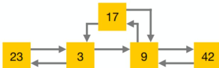
The old link from “3” to “9” is replaced by a link from “3” to “17”.
